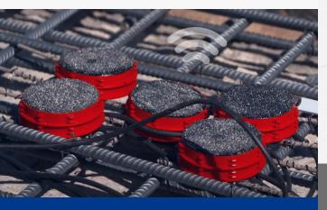
InfrastructureTek uses RFID technology, that once placed inside concrete next to the reinforcing steel, can assess its condition and transmit real-time readings for a lifetime of up to 80 years.
